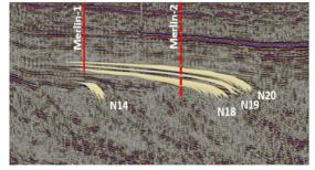
Figure 2: Merlin-2 drilling location and long section showing expected enhanced reservoir thickness to the East
