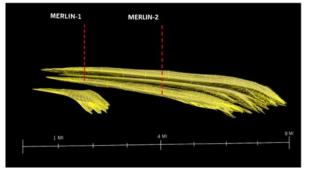
Figure 3: Wireframe image showing respective Merlin-1 and Merlin-2 well locations, facing east and overlain with predicted reservoir sands profile.
