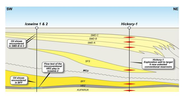
Figure 1: Hickory-1 well designed to test up to 6 stacked targets.
