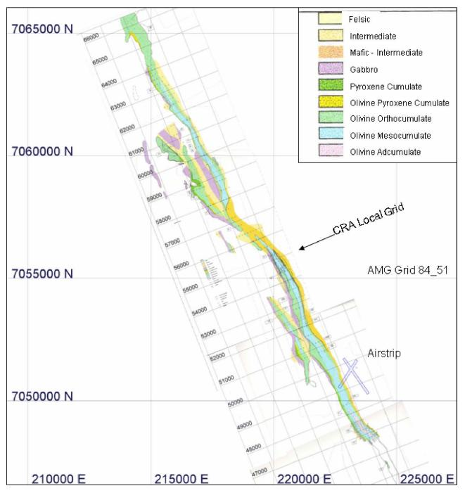
Figure 2: Local sub-surface geology for the Wilconi Ni-Co deposit
