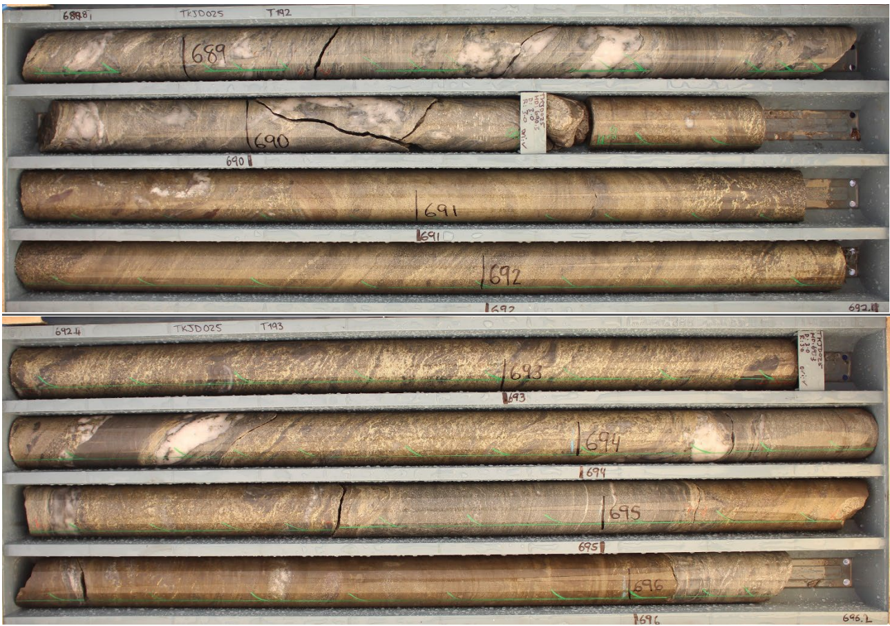
Figure 2 – Core photo from TKJD025 showing a massive to semi-massive sulphide interval from 690.3 metres down hole (assays pending).
