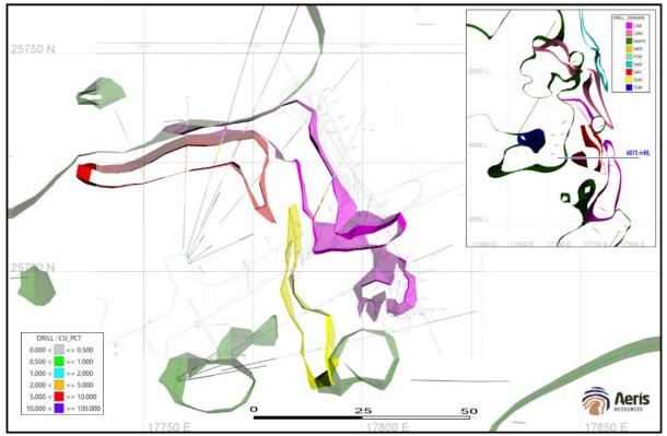
Figure 5 - Plan view of 4875 mRL level showing modelled mineralised solids, mafic volcanics and diamond drilling (Inset shows a cross section at 25,720 mN).
