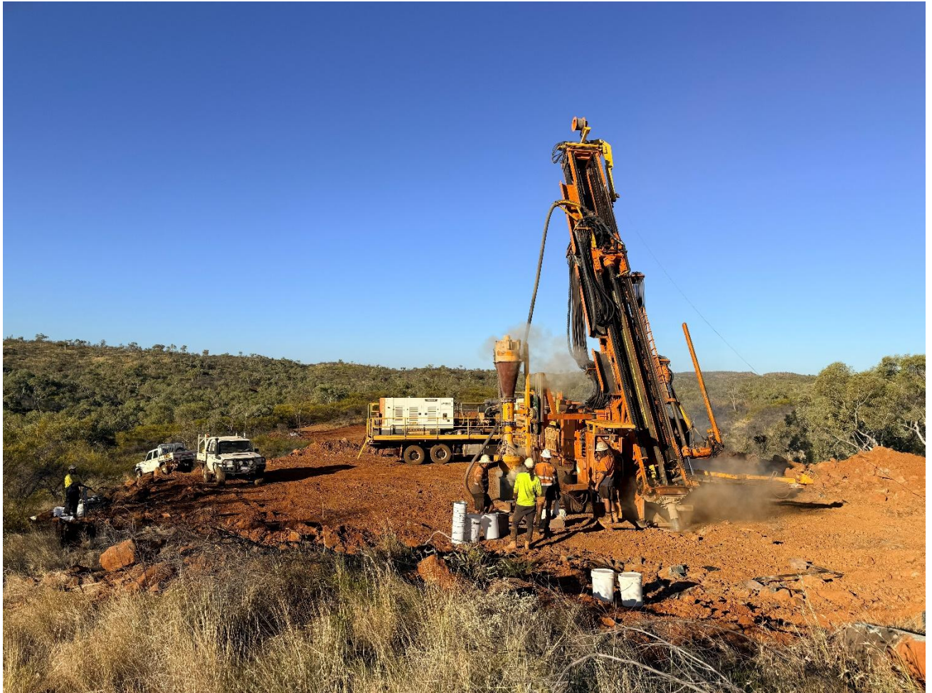
Figure 1: RC drill rig photo from Conglomerate Creek
