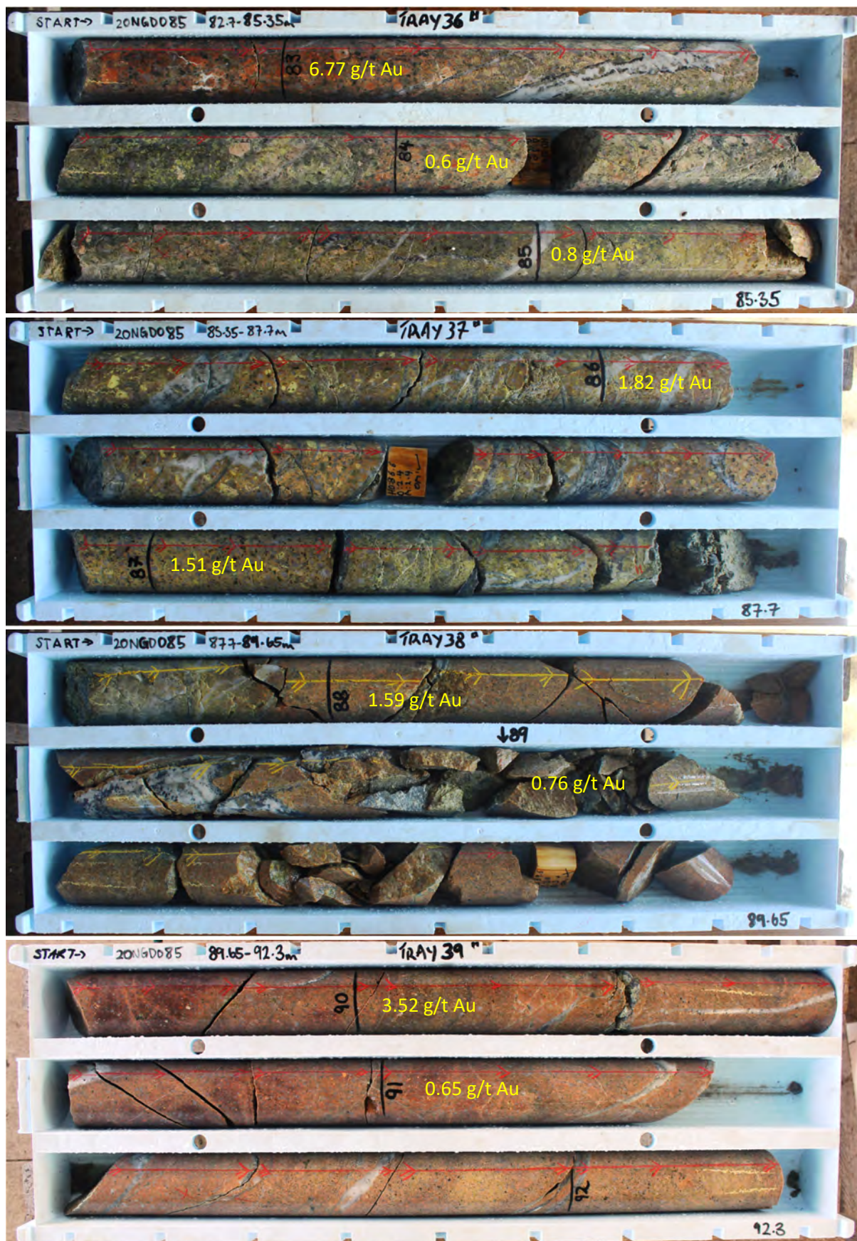
Figure 3 – PQ core trays from hole 20NGD085 – Au grades annotated for 1m half core samples near the start of the interval. Red or yellow arrowed lines on the core are the 'bottom of hole' orientation line.
