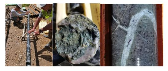
Image 1. (Left) – Cleaning the core at the split tube prior to transfer to core boxes. (Centre) – Core photo at ~190 metres depth, assays awaited. (Right) – Core photo at ~200 metres depth, assays awaited. Core is HQ sized and has a diameter of 63.5mm
