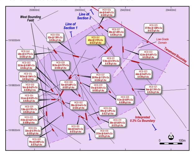
Figure 1. Location of MCB-041 drill hole relative to recent and historical diamond drilling at MCB.
