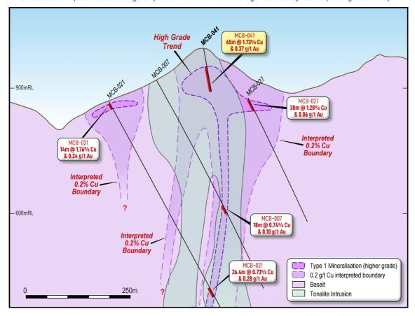
Figure 3. Cross section 2 (see location at Figure 1) of drill hole MCB-041 and significant assay results (looking southwest).
