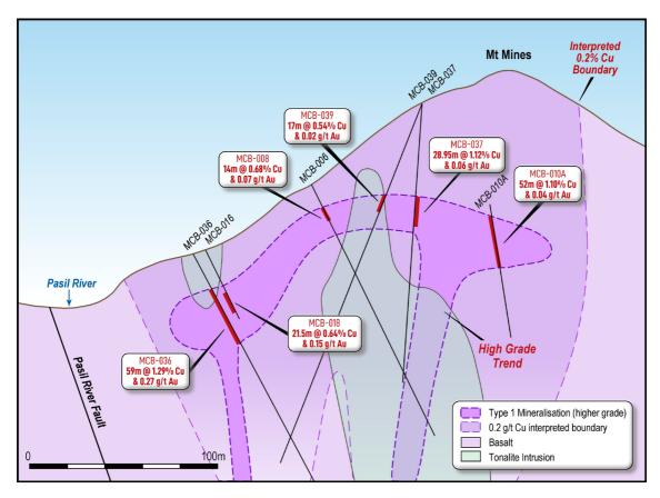
Figure 2. Cross section 1 (see location at Figure 1) of drill hole MCB-041 and significant assay results (looking southwest).
