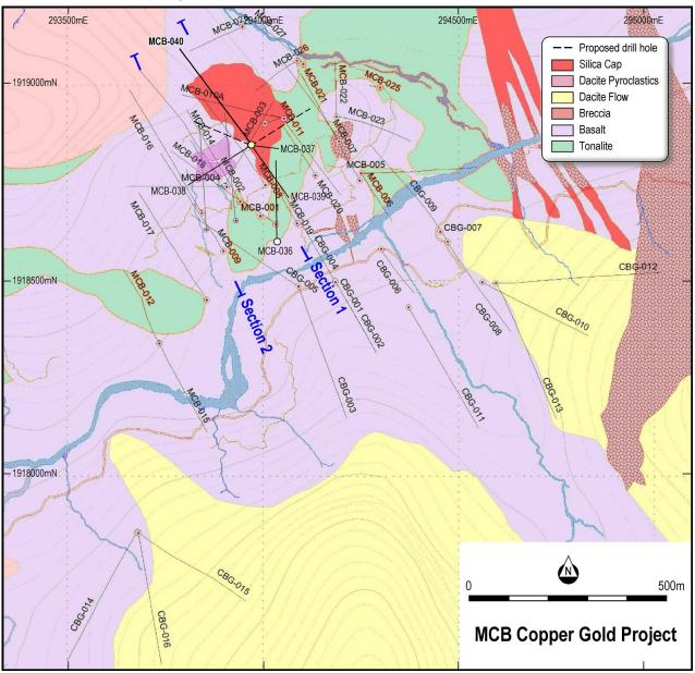
Figure 3: MCB Project drill hole locations and interpreted surface geological plan view diagram.
