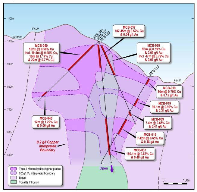
**Figure 4.** Section 1 (see figure 3 for reference location) with the interpreted host rock geology relative to the defined copper mineralised domains. Drill holes completed after the 2020 Mineral Resource estimate on this cross section are identified (MCB-037, MCB-039 and MCB-040). View looking East.
