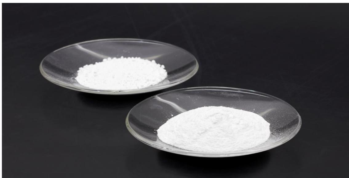
**High purity scandium oxide produced from processing of Syerston ore**
