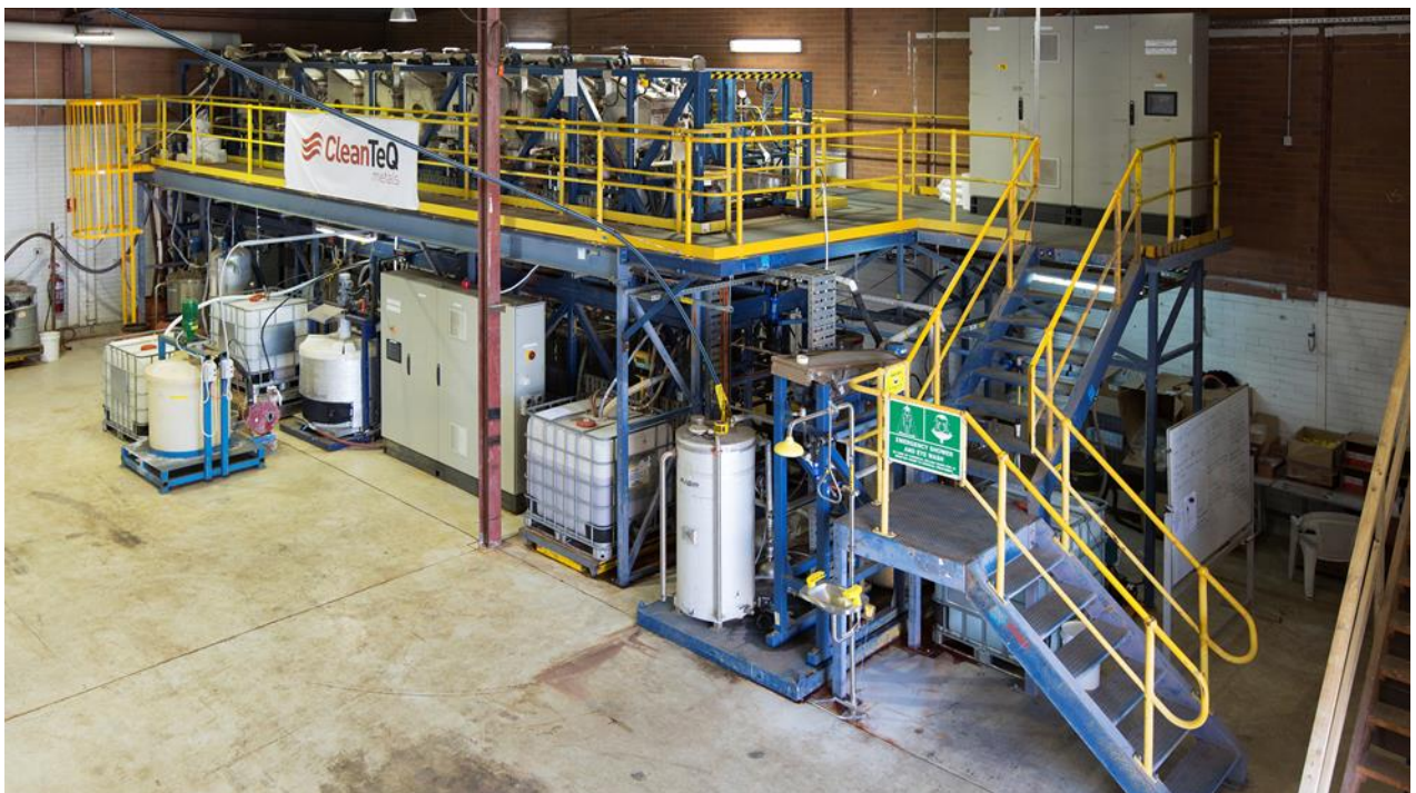
Clean TeQ's proprietary Resin-In-Pulp (cRIP) process demonstration plant
