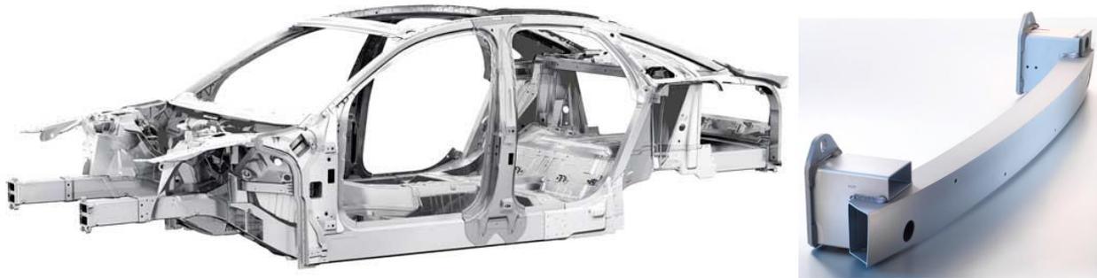
**Figure 4: Body structure<sup>11</sup> and crash management systems<sup>13</sup> produced from aluminium**
