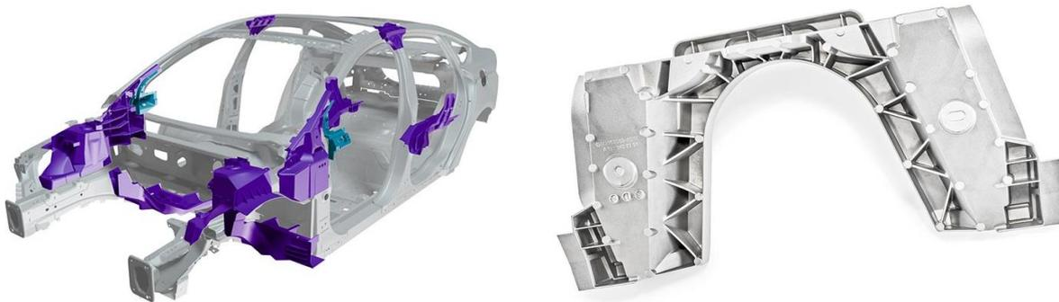
**Figure 6: Aluminium cast parts for automotive<sup>16</sup>**
