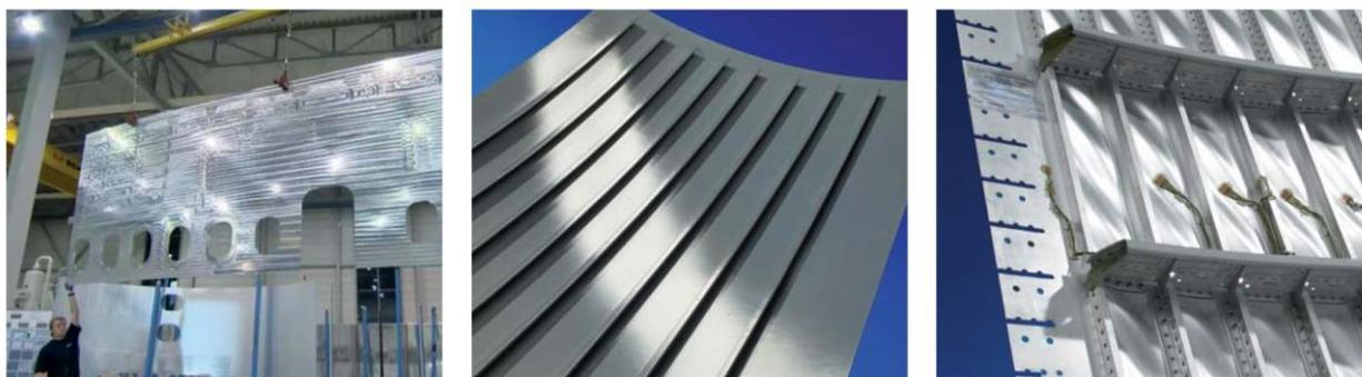
**Figure 2: Aleris creep formed AlMgSc fuselage skin component**
