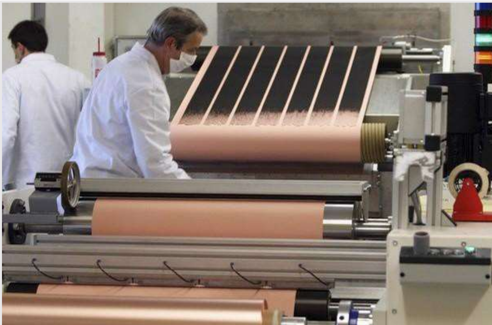
Copper foil used in lithium batteries
