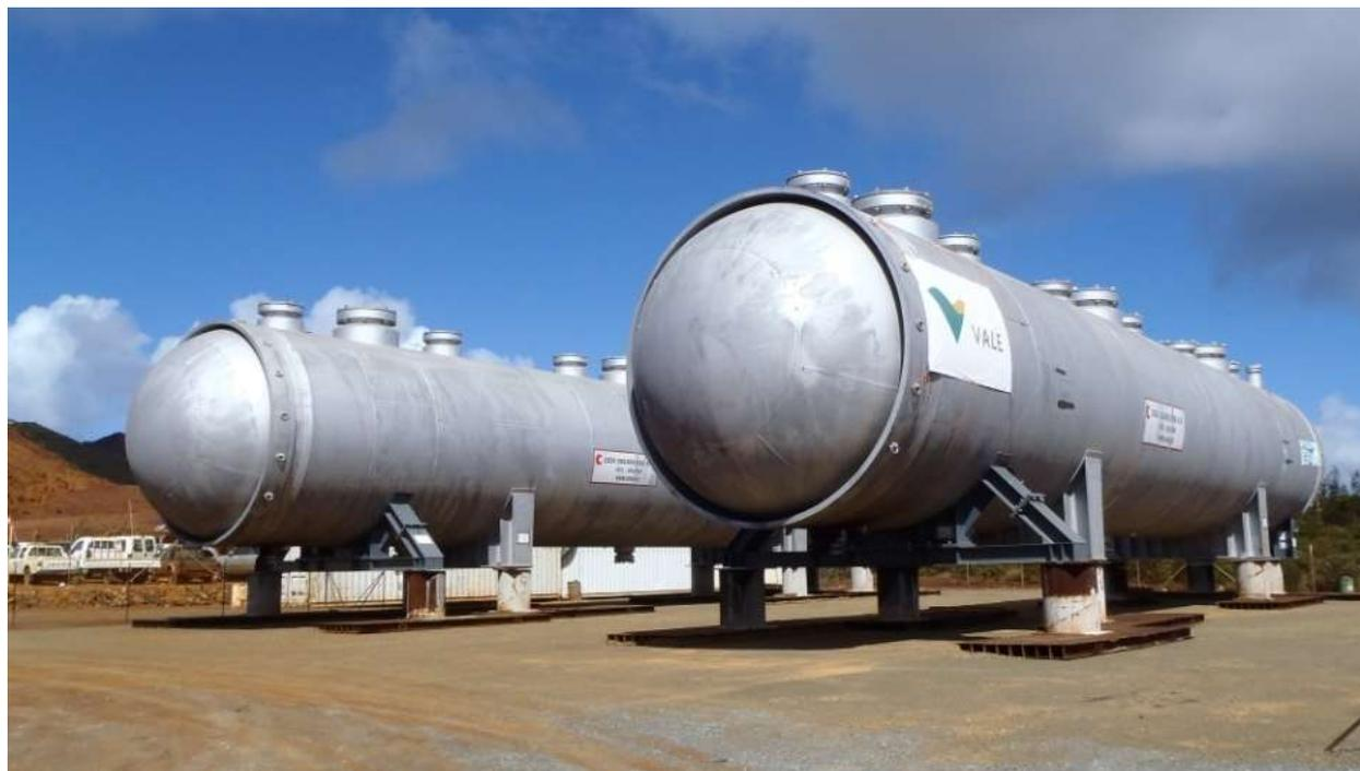
**Figure 2: Autoclave vessel in transit to New Caledonia**
