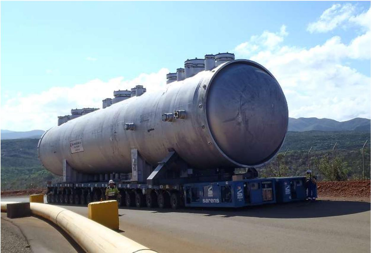
The autoclaves are the major component of the high-pressure acid leach (HPAL) circuit for the Syerston Project. They are pressure vessels with steel shells and explosively bonded titanium lining, which are designed to withstand the operating conditions required for effective leaching of nickel, cobalt and scandium from Syerston ore. The key features of the autoclaves include:
