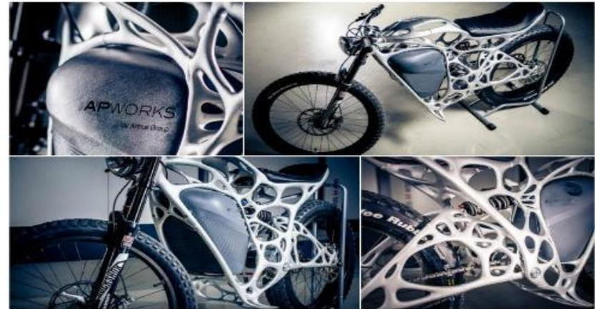
The world's first 3D printed electric bike aluminium-scandium frame makes it lighter and stronger
