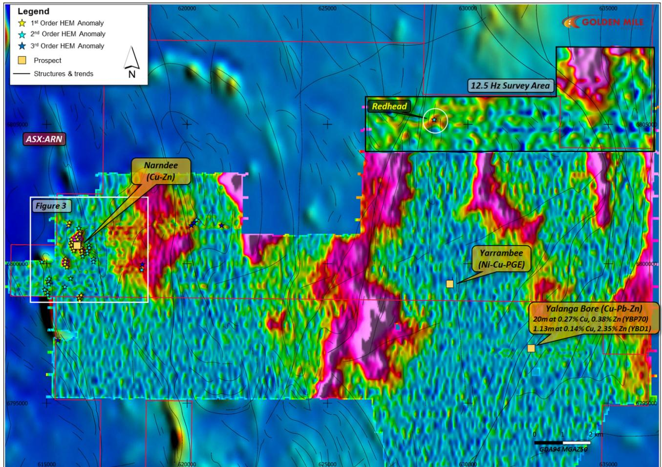
**Figure 2:** Yarrabee HEM survey. Main block image is 25Hz base channel 23 Bfield (Z component). Northeast block image is 12.5Hz base frequency (channel 457 Z component). Background image regional magnetics (RTP-TMI). Areas of broad conductive responses reflect conductive overburden (e.g. saline groundwater).
