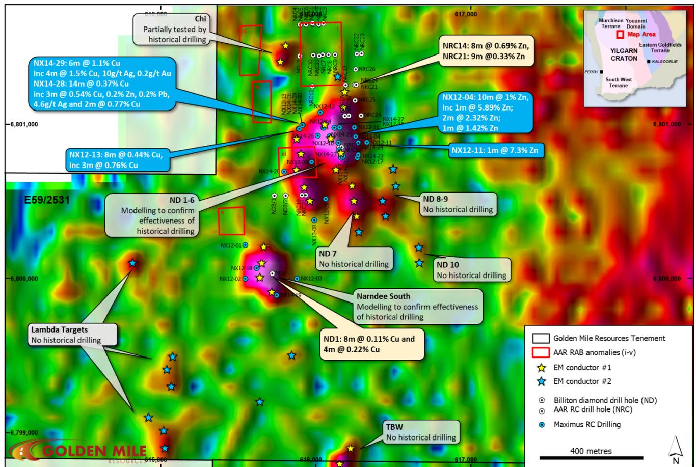
**Figure 3:** Yarrabee HEM survey and base metal targets with historical exploration. Background image is 25Hz base channel 23 Bfield (Z component). Refer body of text for discussion of historical work.
