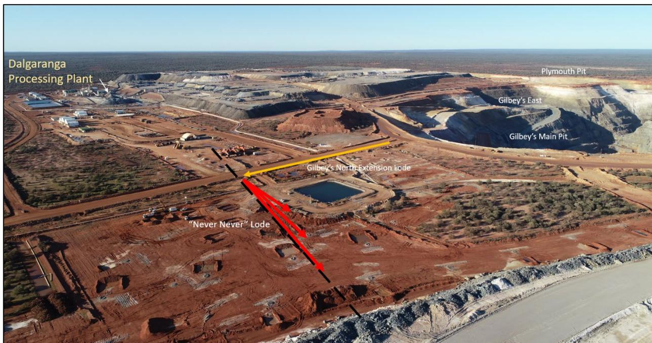
**Figure 4:** Aerial image looking east showing the Gilbey's North Extension Lode in yellow (initial discovery) and the newly defined west-plunging high-grade "Never Never" Lode (red), as well as proximity to nearby infrastructure.
