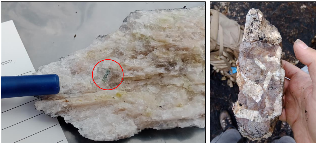
Figure 15 and 16: Left: Pegmatite containing potential beryl (±Apatite?) mineral within Dalmas project (Pen lid for scale, 316859mE, 5943604mN, WGS 84/UTMZ19N), Right: Quartz Feldspathic pegmatite sample taken from Hiver project (302519mE, 5995547mN, WGS 84/UTMZ19N)
