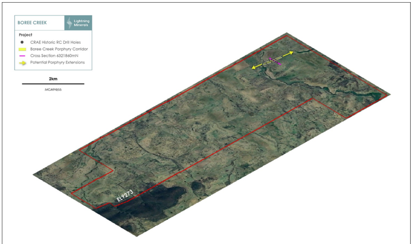
Figure 14: Isometric view of Boree Creek/Dairy Hill Project showing a 700m porphyry corridor open along strike
