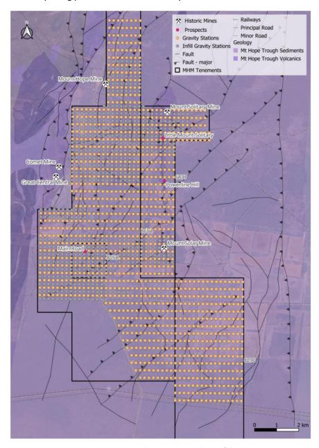
Figure 1: Gravity station locations, including infill stations
