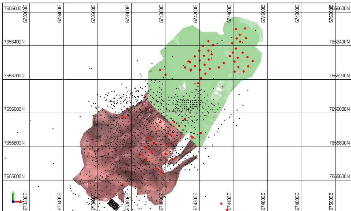
The locations of samples which were re-assayed for Li<sub>2</sub>O are shown in figure 2 below (black), together with the new drill hole sample locations (red).
