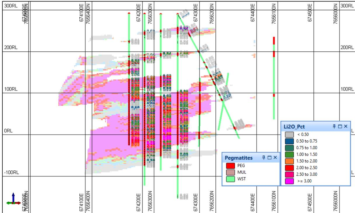
Figure 5 Li<sub>2</sub>O Block Model and Data on Section 20275 North
