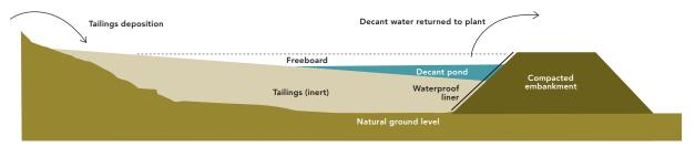
Figure 25: Valley-fill type TSF (TSF3E is an example of this type of facility)
