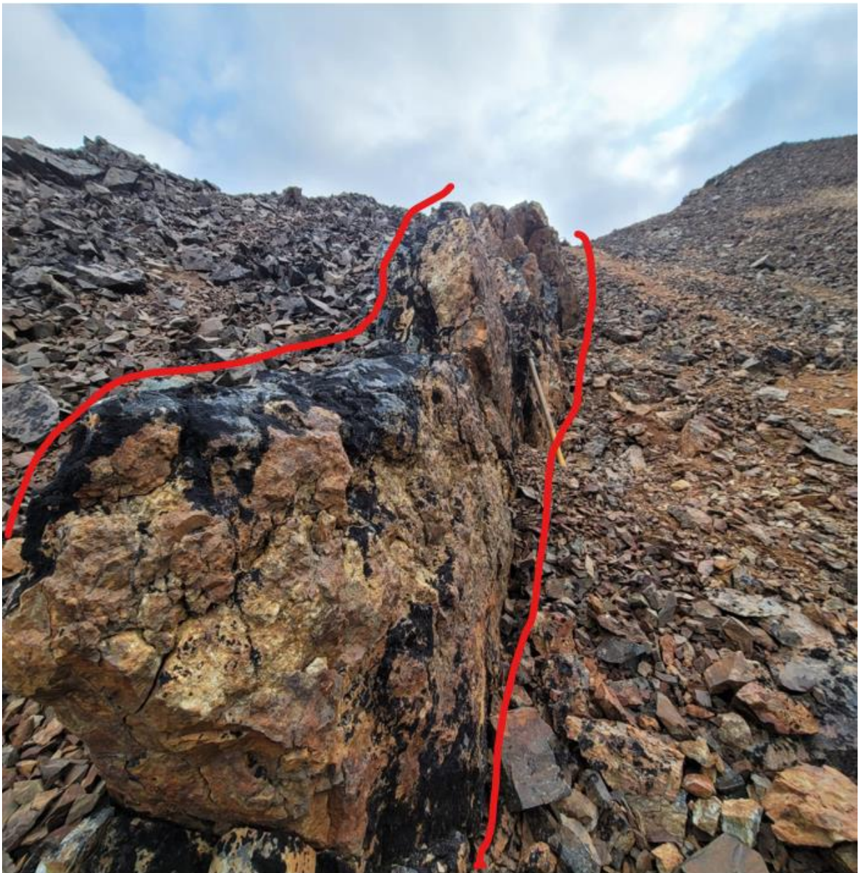
Figure 4. Large vein (~1m thick) strike 088, dip 82 SE containing massive stibnite (~20%) in outcrop at Styx. Stibnite bearing veins are observed in hornfels host rocks in contact with quartz monzonite intrusives.
