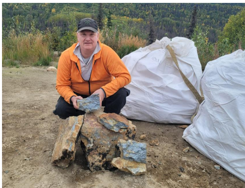
Figure 1. Nova CEO, Mr Christopher Gerteisen at Estelle inspecting potential antimonious bulk samples containing massive stibnite, which are being sent for metallurgical test work.
