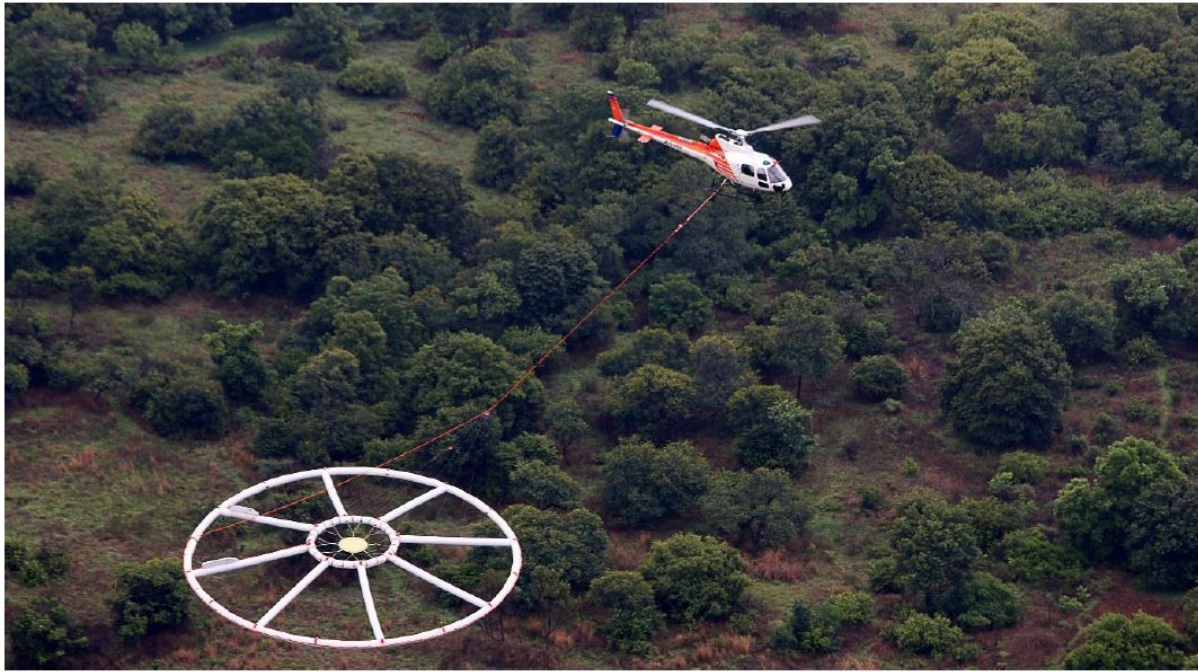
Figure 11: The Xcite airborne electromagnetic and magnetic system collects high-resolution geophysical data for targeting Bali sulphide mineralisation.
