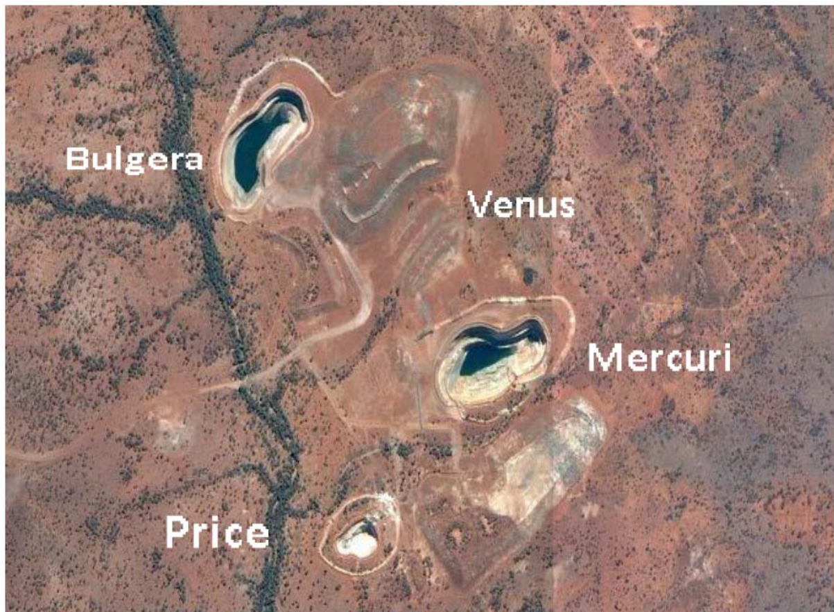
Figure 25 – Shallow open cut mining up until 2004 from Bulgera Gold project (Venus pit backfilled).
