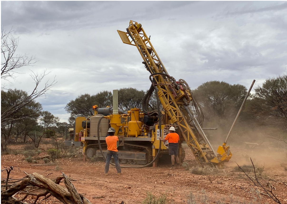
Figure 11 Aircore drilling at the Bulgera Gold Project with track mounted rig capable of RC conversion
