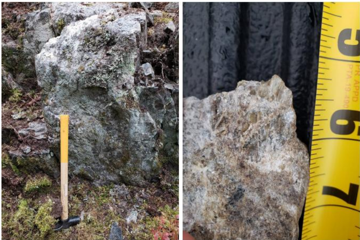
Figure 2: Photo of spodumene bearing pegmatite outcrop hosted within metasediments (left) and medium grained spodumene lathes within a pegmatite sample (right) from the central corridor, mineralised sample returned 2.95% Li 2 O (ASX:PLN 24/10/2023)
