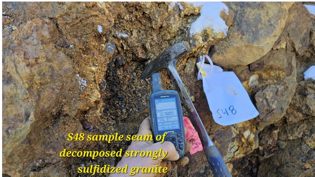
Figure 6: Photo showing sample S48 at Springfield Prospect, here we see strongly oxidised sulphides in granite which returned 7.75 g/t Au and 0.1% WO 3
