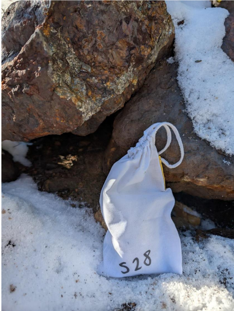
Figure 3: Photo of sample 28 taken from the Springfield Prospect showing massive Pyrrhotite, sample 28 returned WO_3 grades of 0.96% (AS X:PMM 01/12/2025)
