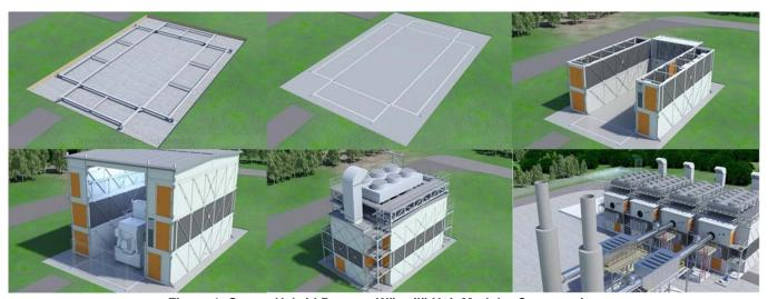
Figure 1: Syama Hybrid Power – Wärtsilä Unit Modular Construction
