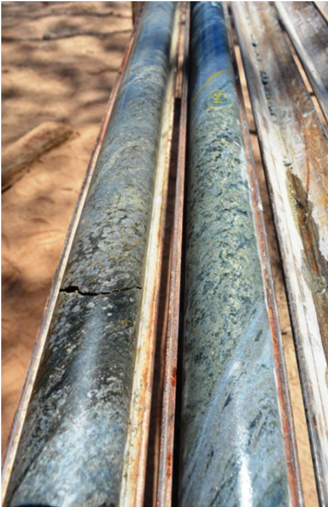
Figure 3 Massive sulphide mineralisation intersected in TH671 with abundant visible sphalerite, chalcopyrite and galena
