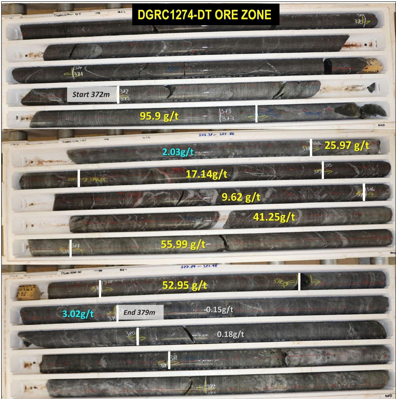
Figure 3: Core photos of drill-core from DGRC1274-DT illustrating “typical” Never Never mineralisation with assay grades overlaid. “Start” to “End”. Note the consistency of high-grade across the 7.00m @ 34.34g/t gold intercept.
