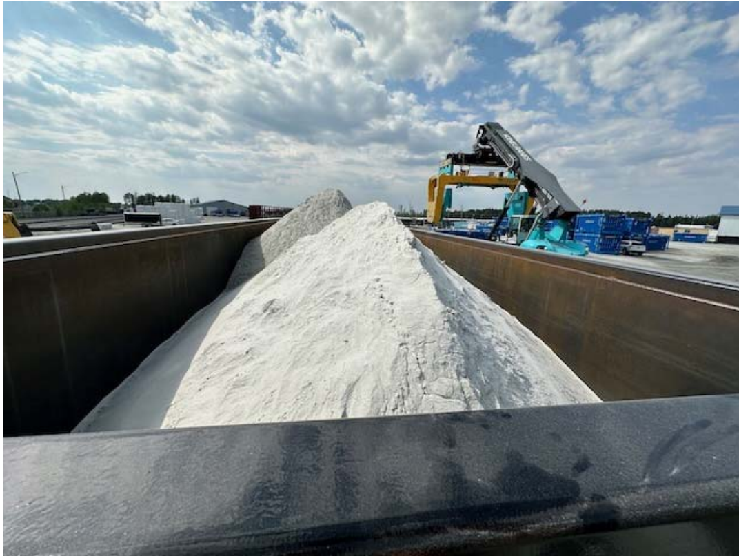
Figure 1: Spodumene concentrate being loaded on rail cars
