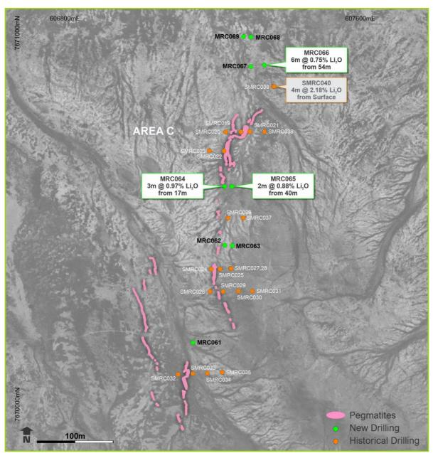
Figure 6: Area C hole plan
