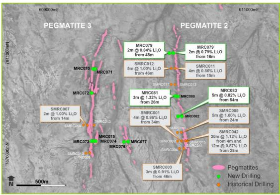
Figure 7: Pegmatite 2 and Pegmatite 3-hole plan showing northward strike extension of Pegmatite 2
