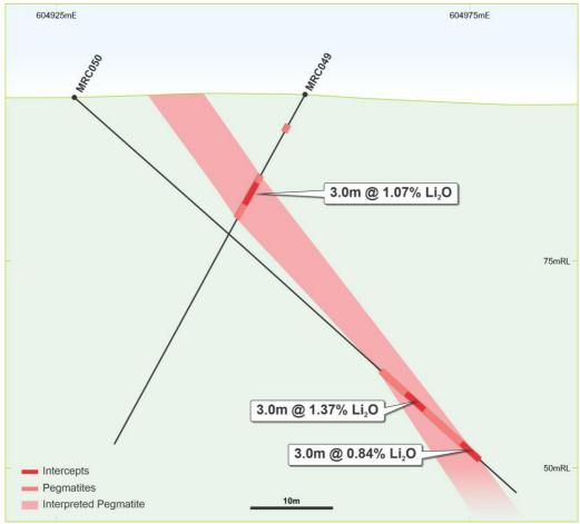
Figure 5: Discovery Section 7671460 showing new intercepts in MRC049 and MRC050
