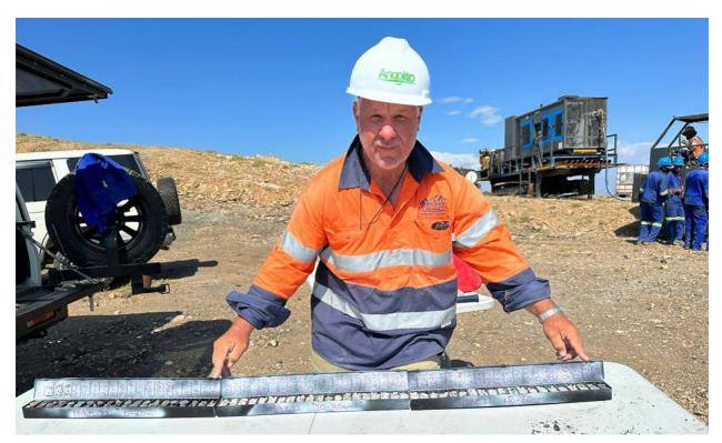
Figure 2: Chip-trays displaying rocks intersected from 0m-60m down-hole of MRC22, with Tyranna Technical Director, Peter Spitalny, indicating the interval of pegmatite from 19m to 59m.
