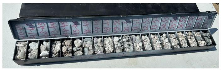
Figure 4: Chip-tray of 40m-60m interval of MRC22. The minerals present include spodumene (10%-20%), lepidolite (1%-5%), elbaite (1%-3%), cleavelandite (variety of albite feldspar, 20%-40%), microcline (variety of potassium feldspar, 5%-10%), muscovite (variety of mica, 5%-10%), and quartz (20%-30%).
