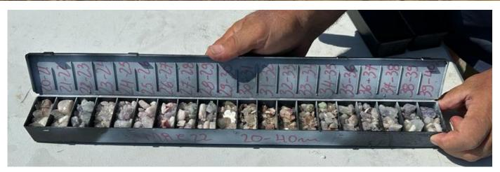
Figure 3: Chip-tray of 20m-40m interval of MRC22. The minerals present include spodumene (10%-20%), lepidolite (1%-5%), elbaite (1%-3%), cleavelandite (variety of albite feldspar, 20%-40%), microcline (variety of potassium feldspar, 5%-10%), muscovite (variety of mica, 5%-10%), and quartz (20%-30%).
