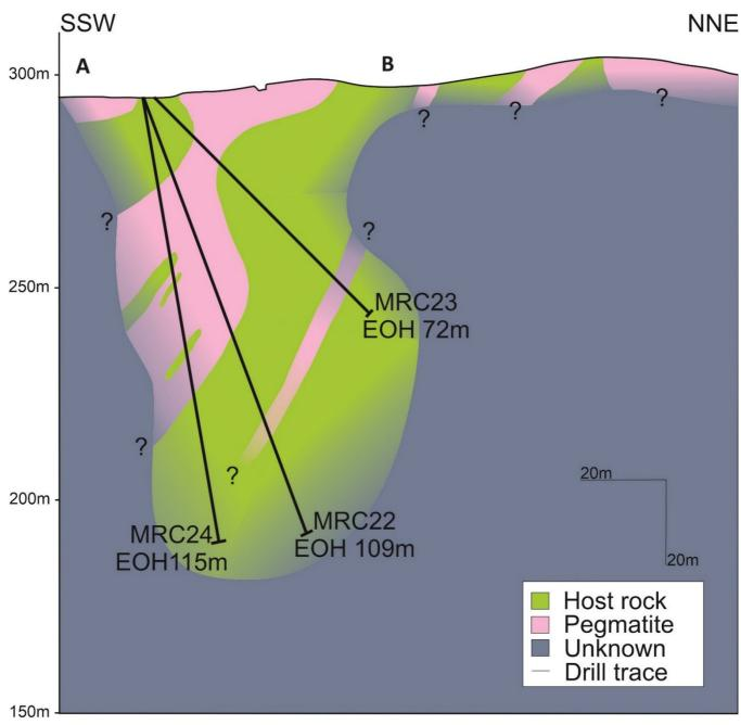
Figure 7: Cross-section A-B, showing interpreted geology intersected by MRC22-MRC24
