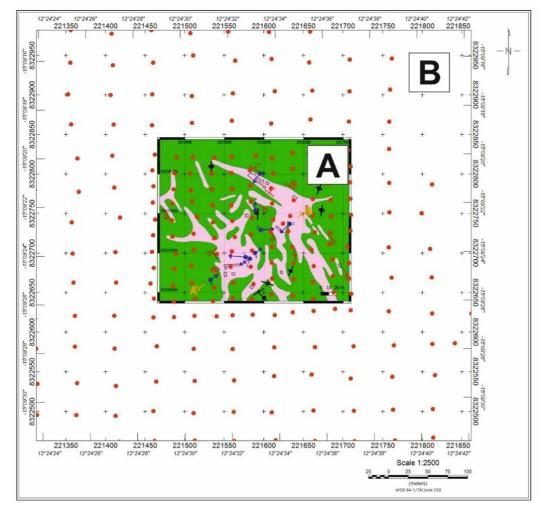
Figure 8: Gravity stations (in red) distributed at intervals of 25 m (A) and 50 m (B). The detailed map of the Muvero region is enclosed. (Source: Figure 1, confidential report from IGME)
