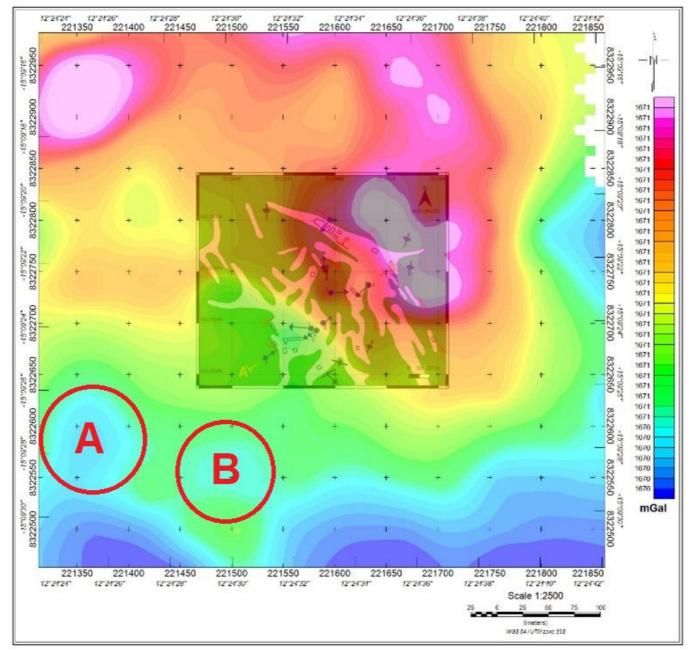
Figure 9: Bouguer anomaly map of the Muvero Prospect, using a density reference of 3.1 g/cm3. Note transparent overlay of part of the pegmatite of the Muvero Prospect, and locations of low-gravity anomalies A and B. (Source: Figure 3, confidential report from IGME).
