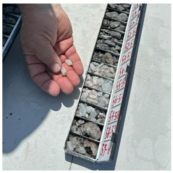
Figure 5: Close-up view clearly displaying spodumene fragments in the 55m-56m and 56m-57m compartments of the 40m – 60m chip-tray of MRC21, and in the hand. Note the mineralisation evident from 54m to 60m, which contains tabular fragments of spodumene (10%-20%), pale blue cleavelandite (variety of albite feldspar, 20%-40%), grey quartz (20%-30%), black tourmaline (1%-5%), microcline (variety of potassium feldspar, 5%-10%) and muscovite (variety of mica, 5%-10%).
