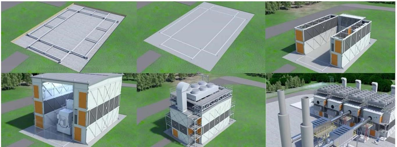
**Figure 1: Syama Hybrid Power – Wärtsilä Unit Modular Construction**
